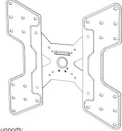
**VERTICAL** supports: 400x400mm 300x400mm 300x300mm 300x200mm 200x400mm 200x300mm
